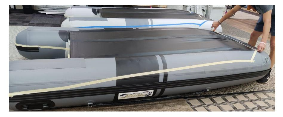
Use the rub rail in the stern as a guide to go around the back of the tubes.
