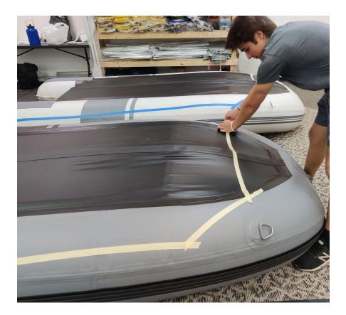
Start by taping across the bow just below where the D-rings sit.
