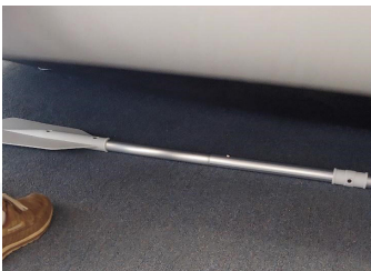
Side View, for larger boats, put 2 oars under the boat, parallel to each other
