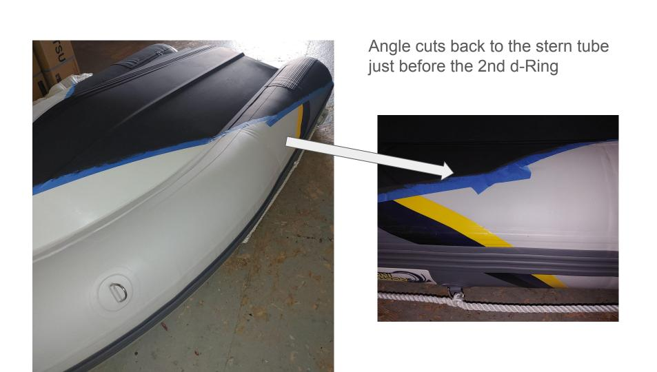
Use the Rub Rail as a guide when you reach the stern cone of the tube to paint the stern where your motor will hang. We suggest painting to just under the lifting eyes across the transom. You can use the same copper-free paint on the tubes and the aluminum hull.
