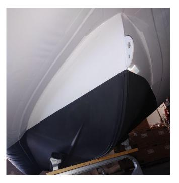
Start from the bow, just under the welded eye in the aluminum hull and angle back to just below the first D-ring
